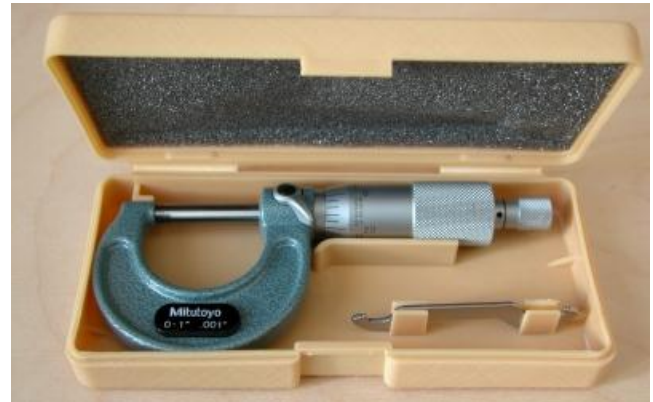
Micrometer -- measures thickness
