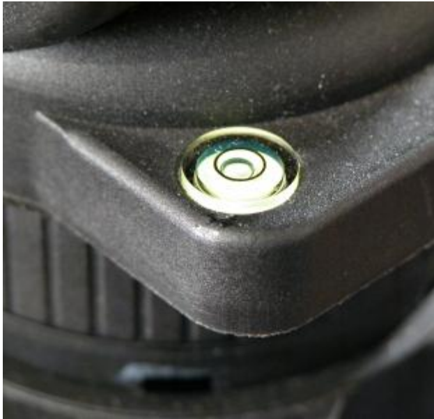
Bubble level as part of the tripod head
