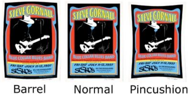
Lens distortion -- barrel and pincushion
